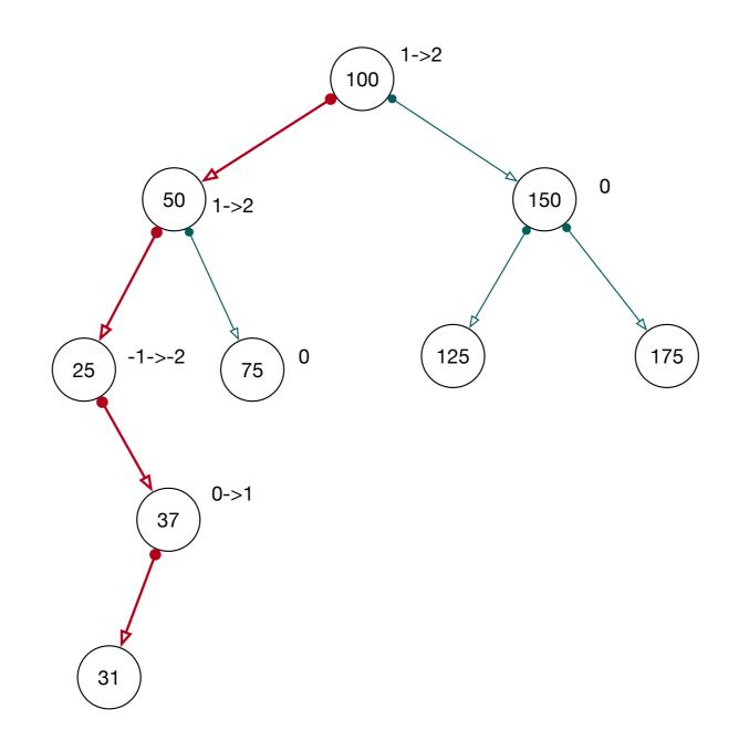
• AVL Insertion: Balances change only on the insertion path
