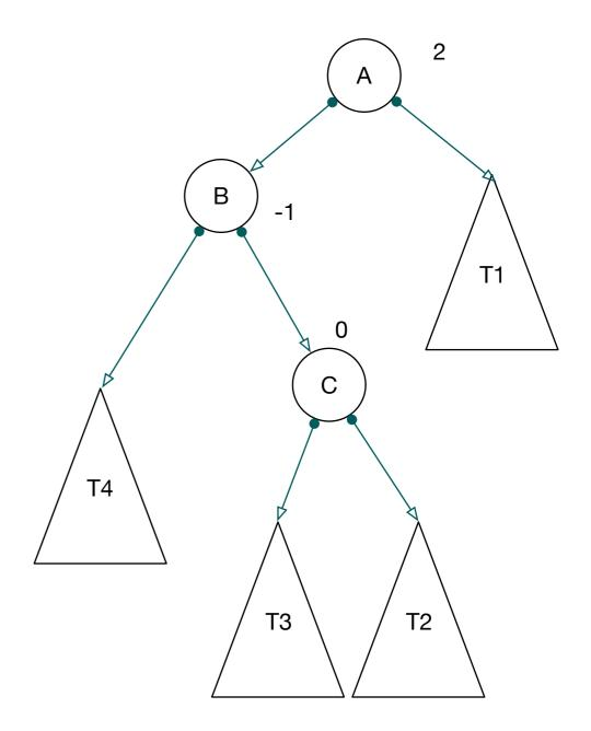
• Double rotate (A with B and B with C)
