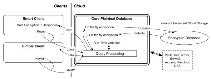
Fig. 1 Reference Architecture of Trusted Cloud DBS
