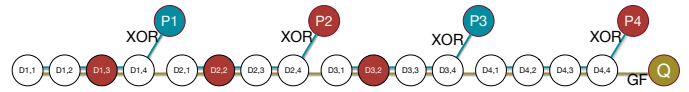
Fig. 2. Reliability stripe with a recoverable pattern of disk failures. Failed disks are shown in red. The P - and Q -parity disks are marked with a letter P or Q , respectively.
