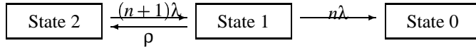
Figure 1: Markov model of a reliability group with n data and one parity bucket.
